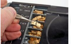
A pair of tweezers was used to pick and place a curved insert into the coder disk.
