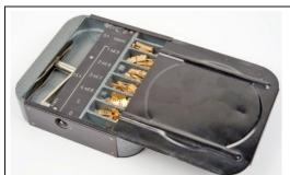
Bottom (storage) compartment of the KSG Geber with bottom lid slid aside showing a pair of tweezers and a crank stowed in the left compartment. In the other compartments were curved metal Morse code inserts.
