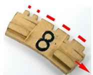
Close-up of a curved insert. The notches at the outer rim represented Morse code number 8 (and number 2 when reversed).
