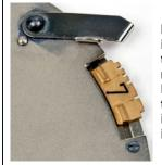
Detail view of loading an insert into the disk which was removed from the KSG Geber during this process. The inserts were placed in reversed order.
